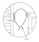
3. Move the furniture to its final position and align the bracket on the furniture with the bracket on the wall. Thread the strap through the bracket as shown, and tighten until snuq. Do not over-tighten.
